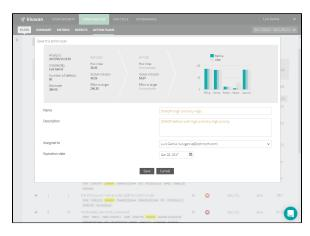
You will see the number of defects contained in this action plan, the effort required to fix them as well as the metrics before and after the fulfillment of the action plan.
