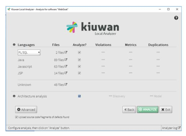
The model will be built when "Architecture analysis" is checked.
